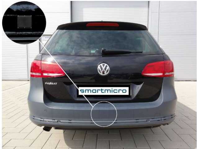
Sensor mounted behind the bumper
