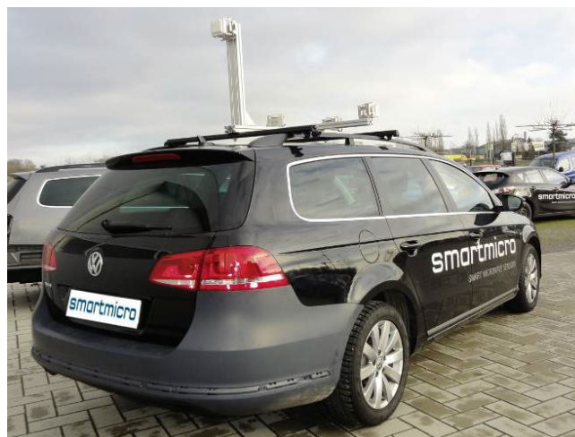
Sensor mounted on top of the car
