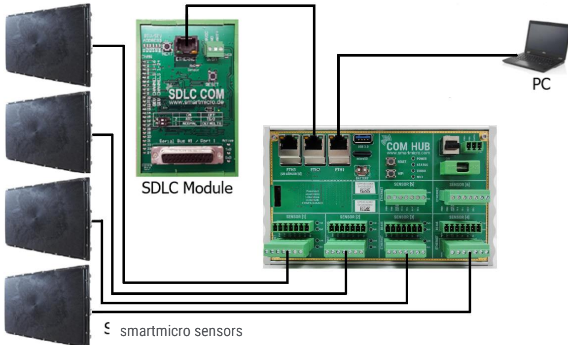
Figure 4-1 Connection with four sensors and COM HUB Sync PLC and SDLC Module
