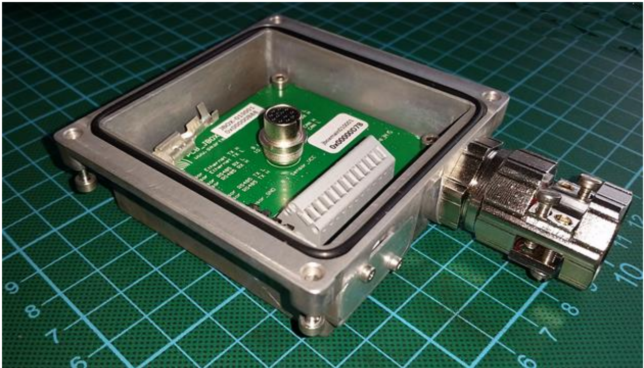
Figure 7: Junction Box JBOX-010001 inner view
