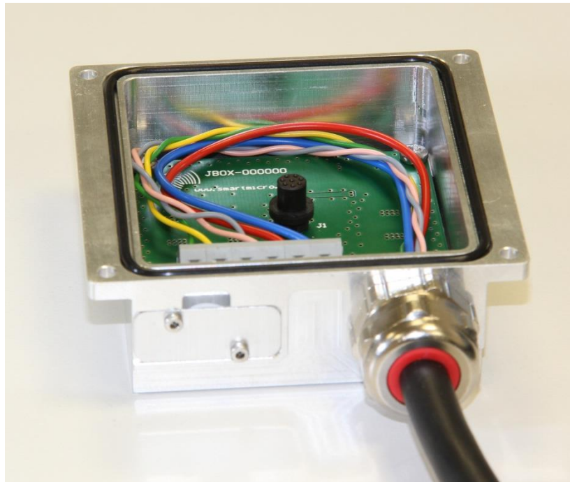
Figure 1: Junction Box JBOX-000000 with attached Lapp cable
