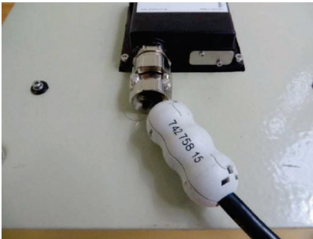
Snap-on ferrite 74275815 on the PLC J-Box side
